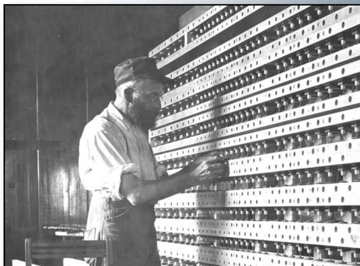
Henry G. Herschler, an important assistant to Abraham Schantz, working on a tubular-pneumatic vent chest in approximately 1906
